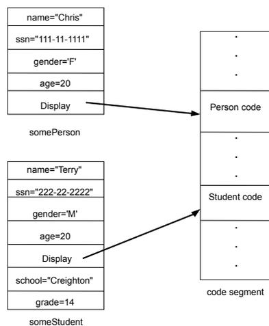
the pointer stores the address of the corresponding code for that class
